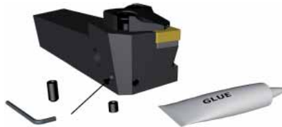
Replace the short screw here with the long screw to shut off underneath coolant
